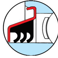
T1000DECG With spherical outside diameter and eccentric collar lock
